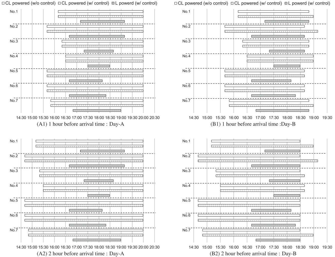
**Fig. 7** Duration of continuous power supply to the critical loads. The computation is conducted with No.1 to 7 data in Table 3 and Day-A or Day-B data in Fig. 4. The figures (A1) and (B1) (or (A2) and (B2)) show the results that commercial power source is tripped 1 hour (or 2 hours) before the arrival time.
