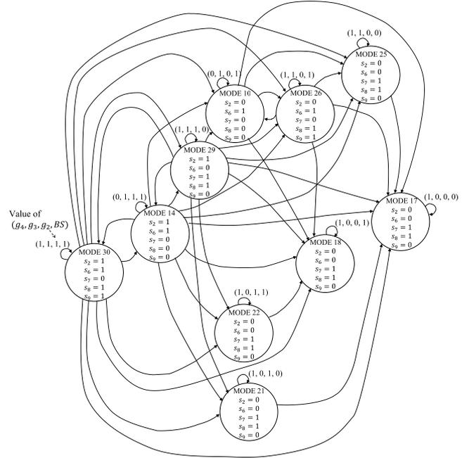
**Fig. 2** Generated automaton of reactive management system under  $g_1 = 0$ . It has the ten control modes determined by the environment variables ( $g_4, g_3, g_2, BS$ ).
