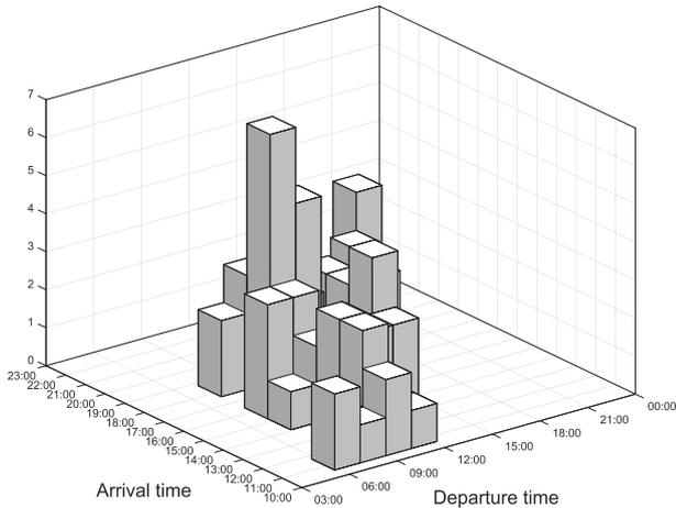
**Fig. 5** Histogram of departure and arrival time for electric vehicles for company use, which is based on the practical measurement in the V2X demonstration project at Osaka, Japan.
