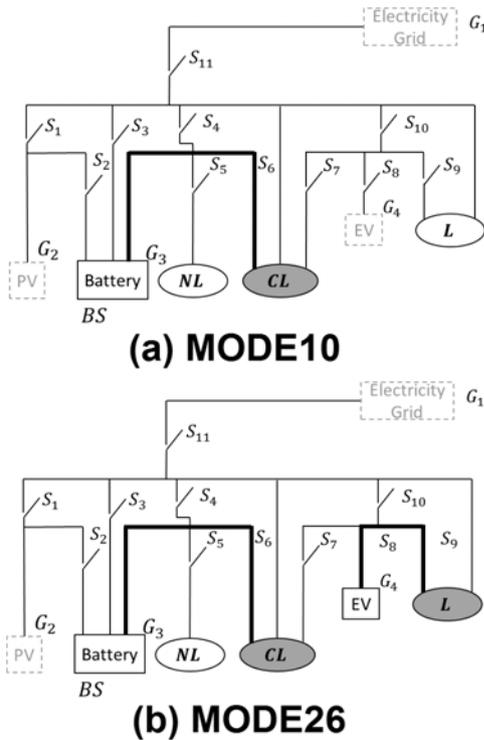
**Fig. 3** Example of control rule of switches shown in Table 2. The *thick* lines represent the synthesized routes of power from source to load. The power sources encompassed by the *dotted* lines are unhealthy. In MODE10, PV  $G_2$  and EV  $G_4$  are unhealthy. Battery supplies power to  $CL$ . In MODE26, both Battery  $G_3$  and EV  $G_4$  are healthy. Thus, Battery supplies power to  $CL$ , and EV does power to  $L$ .
