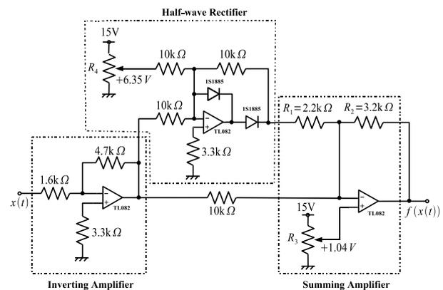
Fig. 11 Nonlinear function circuit.
