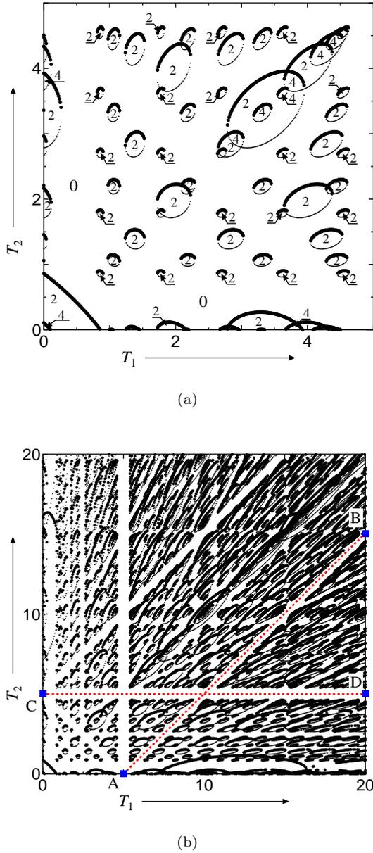
**Fig. 3** Marginal stability curves of  $x^*$  ( $\alpha = 1.0$ ,  $\beta = -3.0$ ,  $\tau = 5.0$ ,  $k \approx -6.4641$ ): (a)  $T_{1,2} \in [0, 5]$ , (b)  $T_{1,2} \in [0, 20]$
