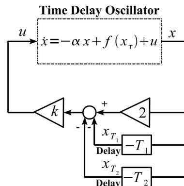
**Fig. 1** Block diagram of multiple delayed feedback control of time-delay oscillators.
