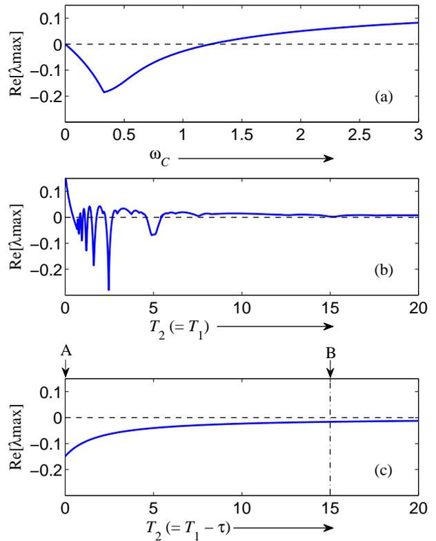
**Fig. 9** Largest real part of the roots  $\text{Re}[\lambda_{\max}]$  of the characteristic equation for the fixed point  $x^*$ : (a) the tracking filter; (b) the original DFC with  $T_1 = T_2$ ; and (c) the MDFC with  $T_2 = T_1 - \tau$ . The parameters are the same as the numerical and experimental results in previous sections ( $\alpha = 1.0$ ,  $\beta = -3.0$ ,  $\tau = 5.0$ ,  $k \approx -6.4641$ ).
