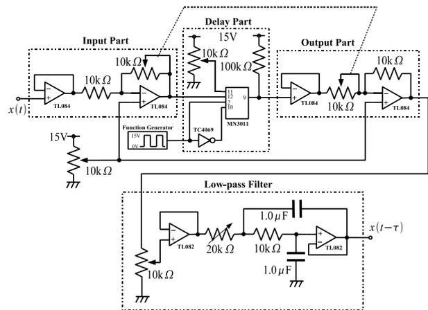
Fig. 10 Delay unit circuit.
