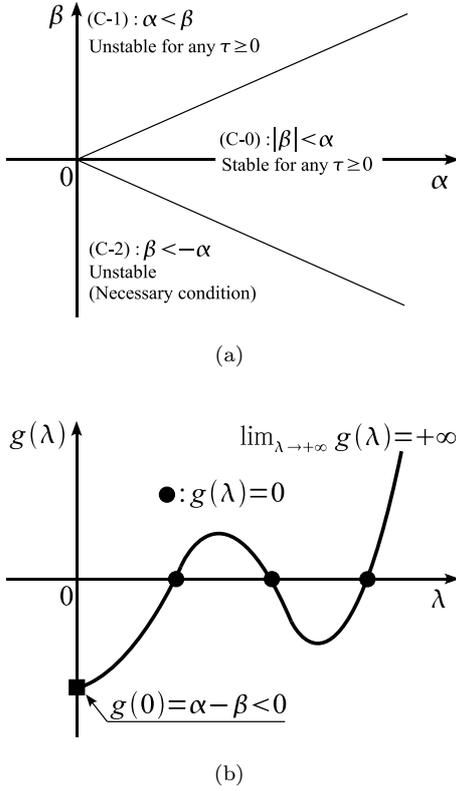
**Fig. 2** Sketches: (a) stability domain of  $x^*$  without control (i.e.,  $T_1 = T_2 = 0$ ) in the  $\alpha$ - $\beta$  plane; (b) function  $g(\lambda)$  with the odd number property.
