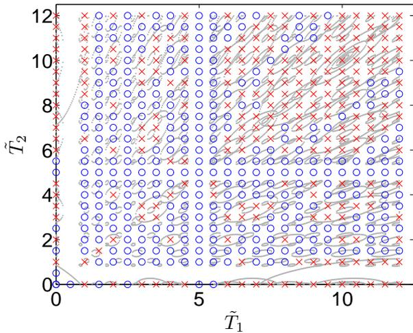
**Fig. 7**  $\tilde{T}_1$ – $\tilde{T}_2$  parameter space for comparison of theoretical and experimental results: the symbol  $\circ$  ( $\times$ ) denotes the occurrence (non occurrence) of stabilization experimentally; the gray lines are the stability curves estimated theoretically.
