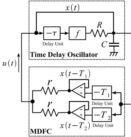
**Fig. 5** Schematic drawing of the time-delay nonlinear oscillator with MDFC.
