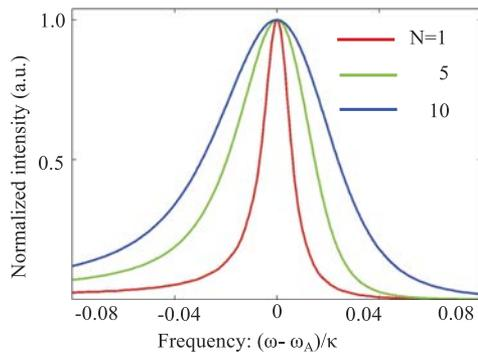
**FIG. 3.** Photoemission spectrum for various numbers of TLSs, namely,  $N = 1$ , 5, and 10. The laser truncation rate is  $\Gamma = 0.8\kappa$ , and the cavity-TLS coupling is  $\sqrt{N}g/\kappa = 0.3$ . The other parameters are the same as those in Fig. 2. Each spectral intensity is normalized by its own peak intensity.
