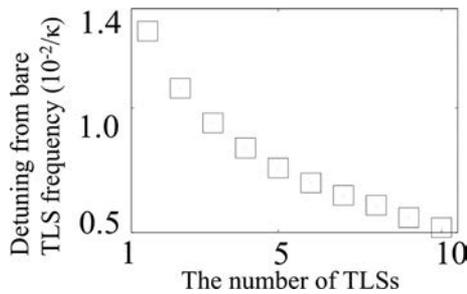
**FIG. 5.** Numerical computation results for the up-converted peak frequencies detuned from an undressed TLS frequency as functions of  $N$  for  $N = 1-10$ .
