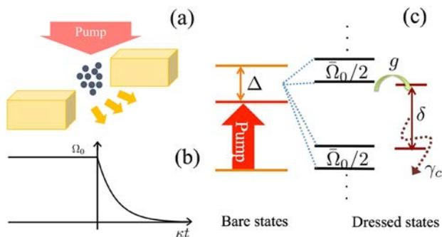
**FIG. 1.** (a) Schematic picture of an ensemble of TLSs in the bad-cavity limit. (b) Temporal profile of the pump light intensity. (c) Level diagrams for the undressed states and dressed states.  $\Delta$  and  $\delta$  denote the TLS detuning and cavity detuning from the driving frequency, respectively.  $\tilde{\Omega}_0 = \sqrt{\Delta^2 + \Omega_0^2}$  and  $\gamma_c = g^2/\kappa$  are the Rabi splitting energy at  $t = 0$  and the cavity-modified decay rate of the TLS, respectively.
