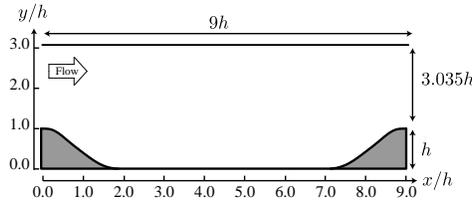
Figure 13: Computational geometry of channel with streamwise periodic hill.
