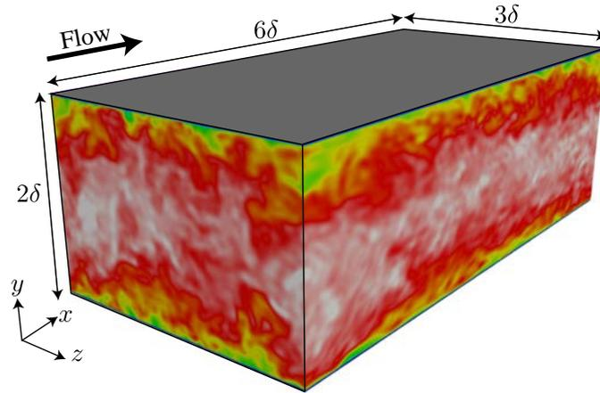
Figure 4: Computational domain of a turbulent channel flow.
