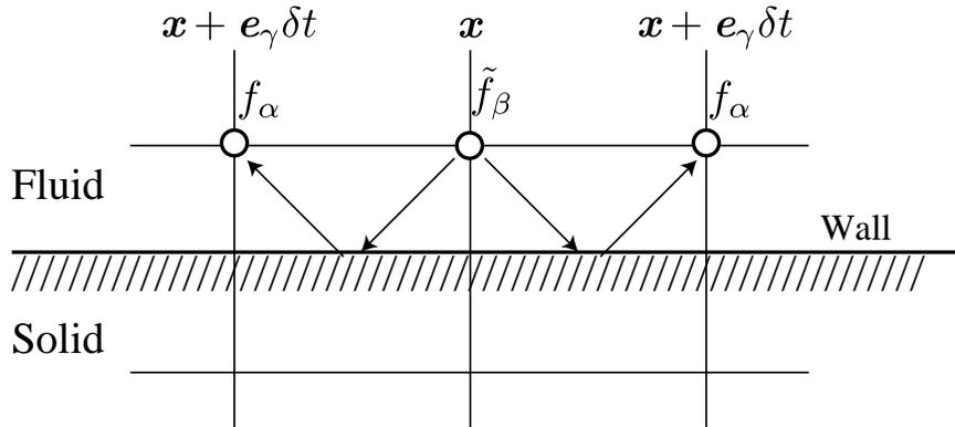
Figure 2: Specular reflection rule.
