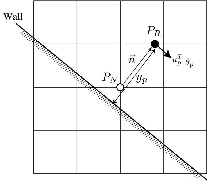
Figure 1: Reference point  $P_R$  for the wall-function method.
