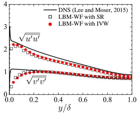
Figure 7: Comparison of the streamwise and wall-normal Reynolds stresses with the DNS data from [52].
