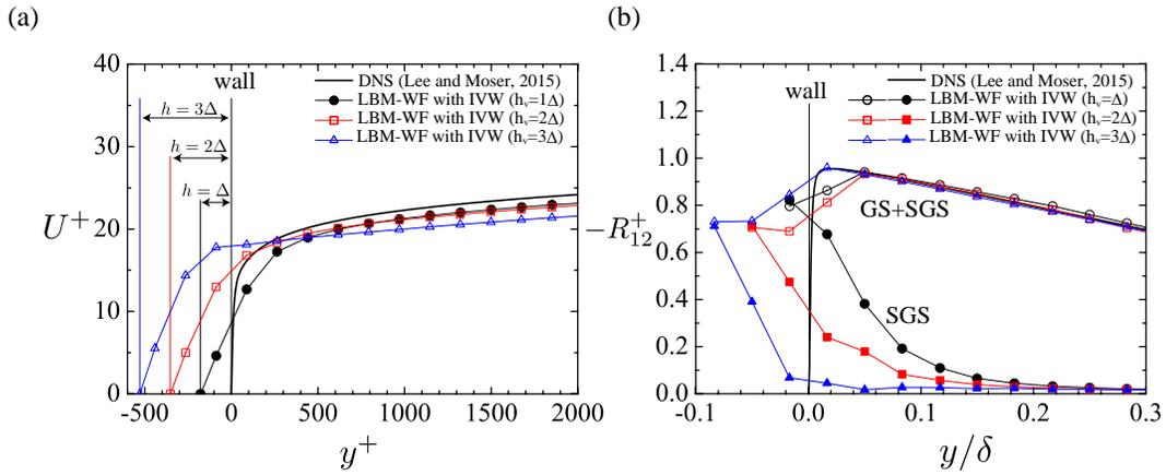
Figure 10: Effect of the virtual wall layer thickness on the predictive results: (a) streamwise mean velocity and (b) Reynolds shear stress profile.
