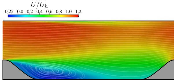
Figure 14: Contour map of the streamwise mean velocity with streamlines.
