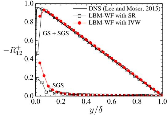
Figure 6: Comparison of the Reynolds shear stress profile with the DNS data from [52]: the SGS (modeled) component,  $2\nu_{SGS}S_{12}$ , and the sum of the GS (resolved) and SGS components,  $-\overline{u'v'} + 2\nu_{SGS}S_{12}$ , are presented.
