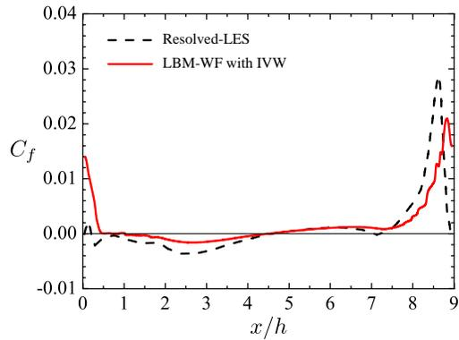
Figure 15: Comparison of the skin friction coefficient with the resolved LES data from [57].
