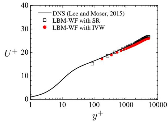
Figure 5: Comparison of the streamwise mean velocity profile with the DNS data from [52].
