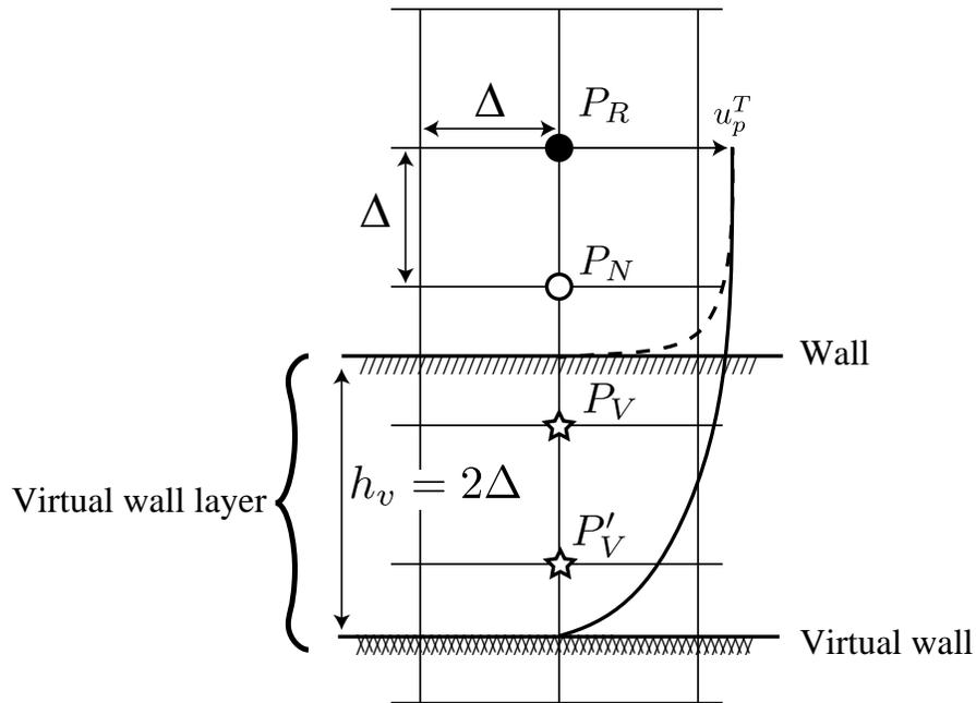
Figure 3: Near wall node points for the immersed virtual wall method:  $P_R$  is the reference point for the wall-function,  $P_N$  is the node neighboring to the wall,  $P_V$  is the virtual node, and  $P'_V$  is the nodes neighboring to the virtual wall. The solid and broken lines are respectively the actual velocity profile and approximated profile by the wall-function.
