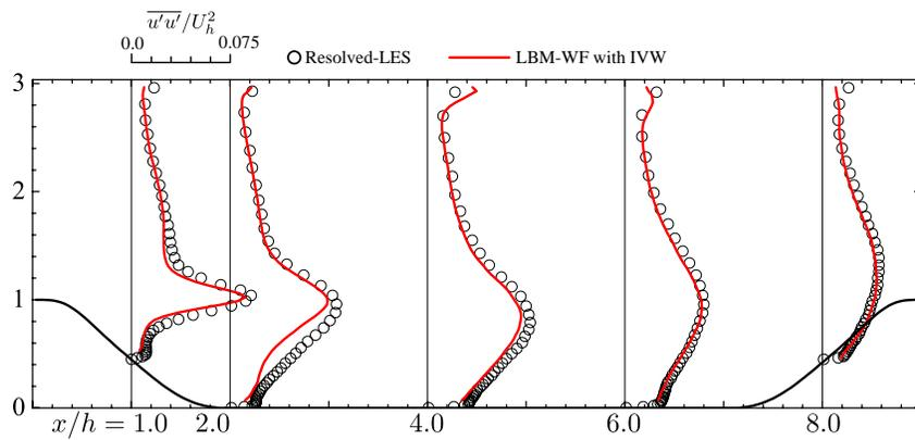
Figure 17: Comparison of the streamwise Reynolds stress profile with the resolved LES data from [56].
