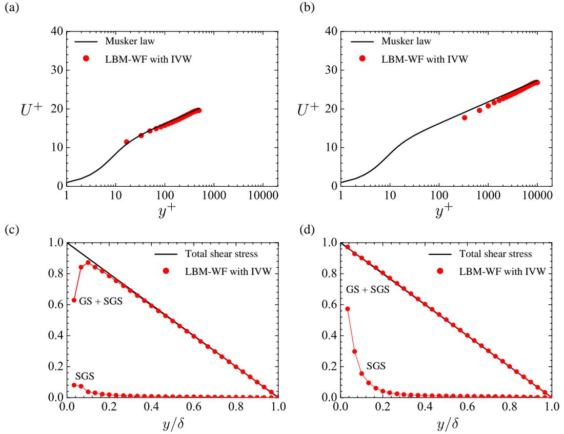
Figure 9: Comparison of the predictive results for different  $Re_\tau$ : (a) streamwise mean velocity at  $Re_\tau = 500$ , (b) streamwise mean velocity at  $Re_\tau = 10,000$ , (c) Reynolds shear stress at  $Re_\tau = 500$ , and (d) Reynolds shear stress at  $Re_\tau = 10,000$ .
