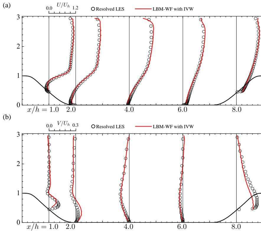
Figure 16: Comparison of the mean velocity profile with the resolved LES data from [56]: (a) Streamwise mean velocity and (b) vertical mean velocity.
