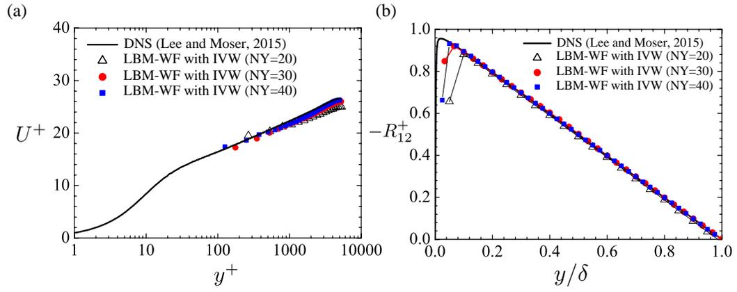
Figure 8: Grid dependence on the predictive results: (a) streamwise mean velocity and (b) sum of GS and SGS Reynolds shear stress.
