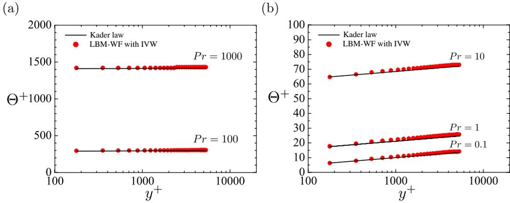
Figure 11: Comparison of the mean temperature profiles for different Prandtl number, (a) for  $Pr = 1000$  and  $100$ , (b) for  $Pr = 10, 1.0$  and  $0.1$ .
