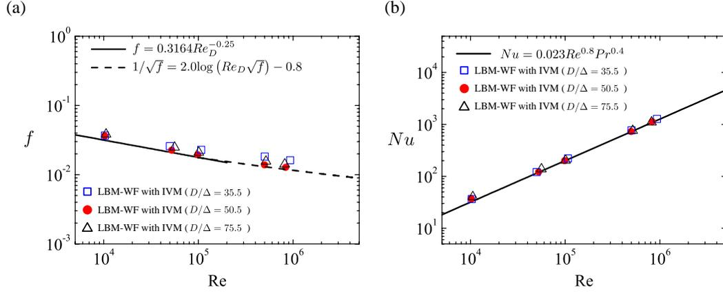
Figure 12: (a) comparison of the friction factor of the circular pipe with  $f = 0.3164Re_D^{-0.25}$  ( $Re_D < 10^5$ ) by [53],  $1/\sqrt{f} = 2.0 \log(Re_D \sqrt{f}) - 0.8$  ( $10^5 < Re_D$ ) by [54], (b) Comparison of the Nusselt number of the circular pipe with  $Nu = 0.023Re^{0.8}Pr^{0.4}$  by [55].
