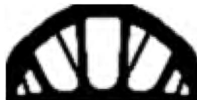
Fig. 8 Optimal configurations of the bridge example
