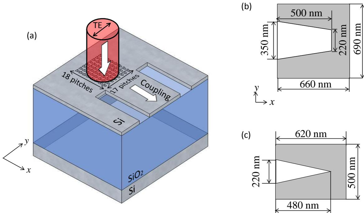
**Fig. 1.** A hole-array grating coupler between a vertically mounted optical fiber and a silicon slab waveguide on a SOI substrate. The grating coupler consists of a two-dimensional array of through-holes in the top silicon layer with a thickness of 250 nm. (a) Unit cell of the optimally designed trapezoidal-hole array. (b) Unit cell of the optimally designed triangle-hole array. These unit cells were designed for the infinitely thick BOX layer.
