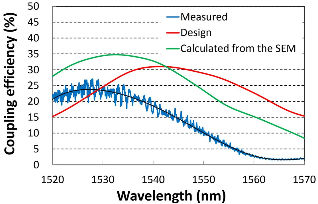
**Fig. 6.** Measured coupling efficiency as a function of wavelength. The measured maximum efficiency was 24% at a wavelength of 1528 nm. The red curve is the calculated efficiency of the optimized design for the 3.0- $\mu\text{m}$ -thick BOX layer. The green curve is the efficiency calculated from the hole-size and pitches acquired from the SEM image of the fabricated grating.
