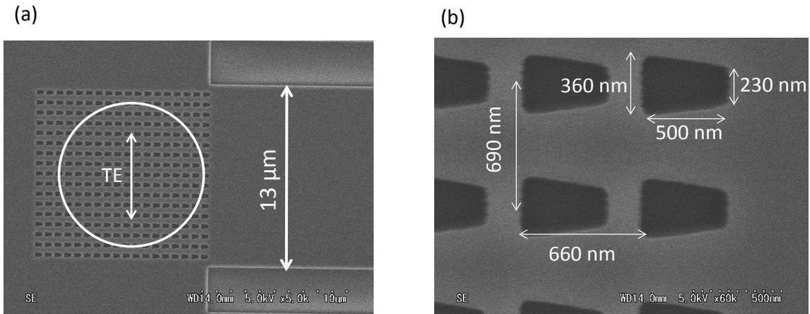
**Fig. 5.** Scanning electron micrographs of the fabricated trapezoidal-hole grating coupler. (a) The grating coupler with a 13 μm wide slab waveguide. The grating consists of 18×17 holes. The white solid circle indicates the core size of the input optical fiber. (b) Enlarged views of the trapezoidal holes. The hole sizes were acquired from the micrograph.
