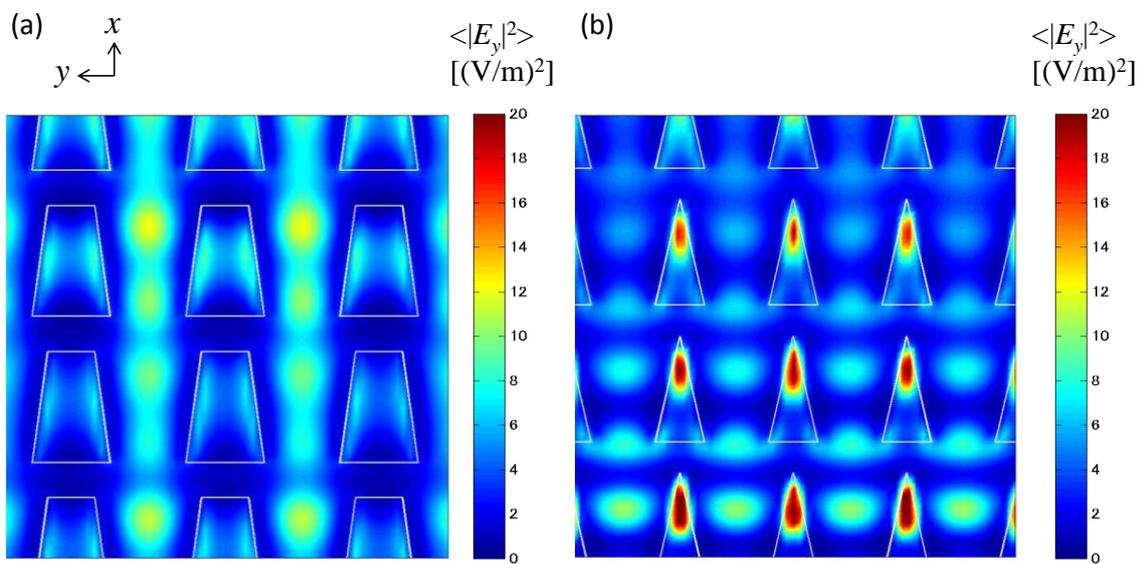
**Fig. 3.** Calculated distributions of the time-averaged square of  $y$ -component of the electric fields in the gratings. (a) The trapezoidal hole array, and (b) the triangle hole array.
