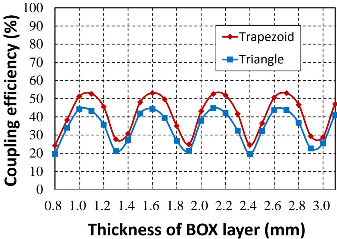
**Fig. 4.** Calculated coupling efficiencies as a function of thickness of the BOX layer for the optimized trapezoidal-hole array and the triangle-hole array. The wavelength of the incident light is 1550 nm.
