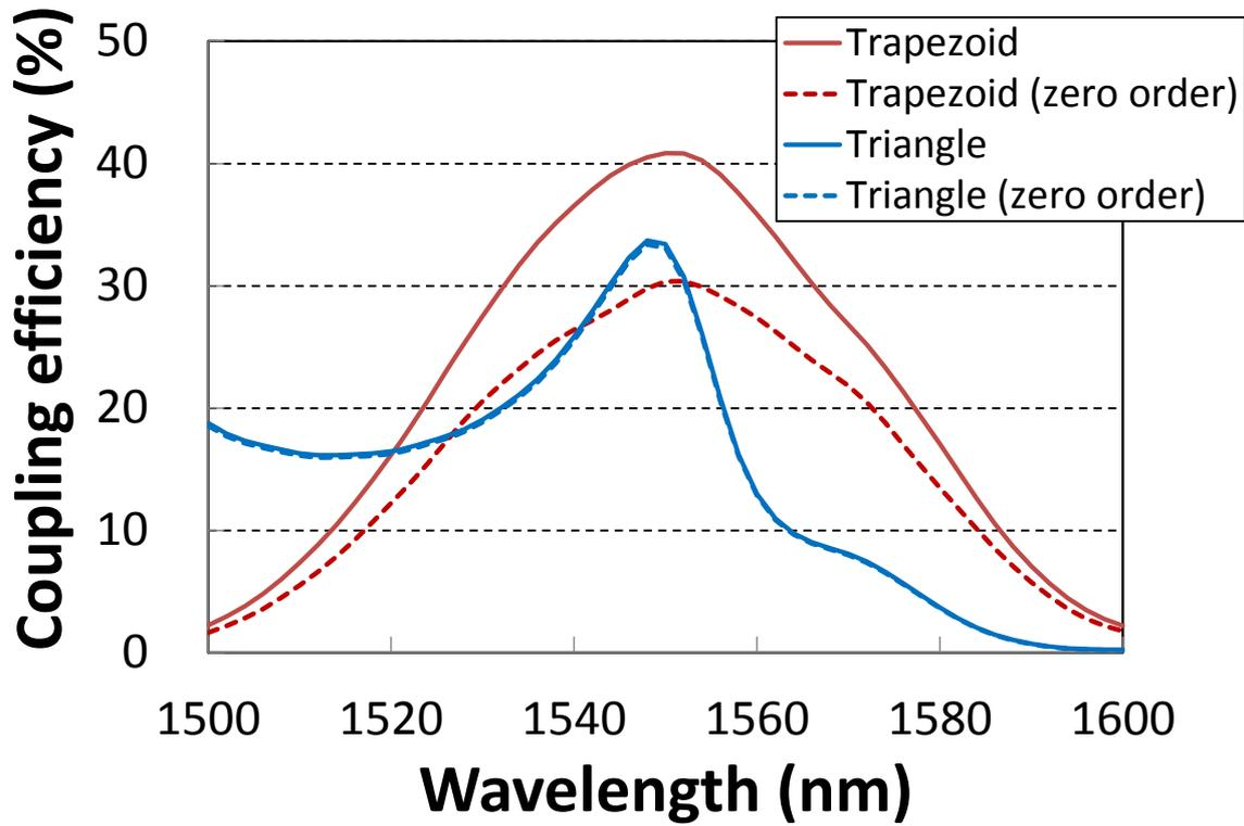
**Fig. 2.** Calculated coupling efficiencies as a function of wavelength of the incident light for the optimized trapezoidal-hole array and the triangle-hole array. Dashed curves are calculated coupling efficiencies only for the zero-order diffracted waves.
