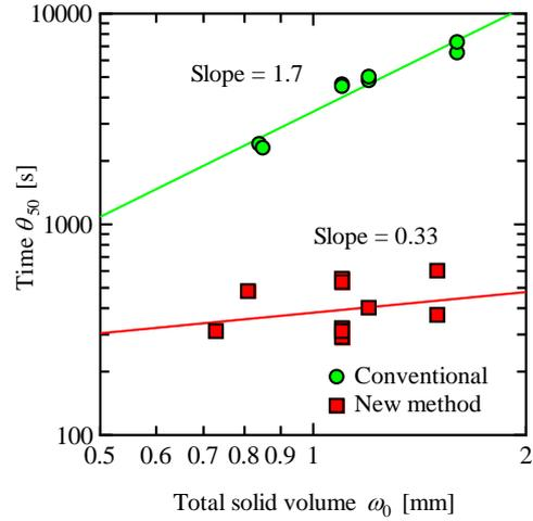
Fig. 3 Effect of  $\omega_0$  on dewatering time  $\theta_{50}$  ( $N = 1500$  rpm).
