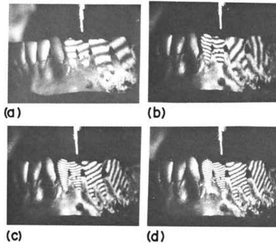
**Fig. 3** Reconstruction patterns obtained from real time holographic interferograms for four different loads, 61 gf, 196 gf, and 216 gf, respectively. (a) 61 gf, (b) 176 gf, (c) 196 gf, and (d) 216 gf.
