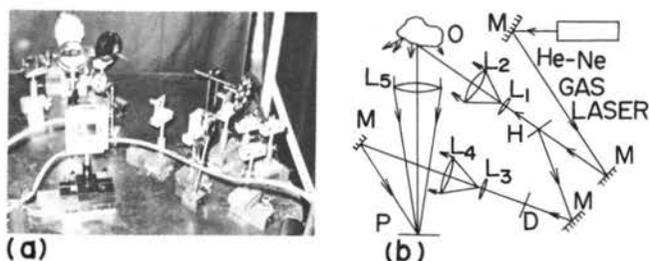
**Fig. 2.** Optical system. (a) Experimental apparatus, (b) Schematic drawing of optical system. M; surface mirror,  $L_1$ ,  $L_3$ ; objective lens,  $L_2$ ,  $L_4$ ; collimating lens, D; density filter, P; photographic plate, O; object, H; half mirror,  $L_5$ ; Fraunhofer lens.
