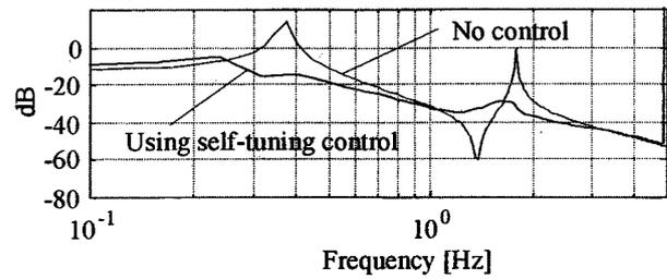
Fig. 15 Frequency response when mass at the tip is increased
