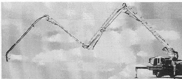
Fig. 1 Concrete distributor arm
