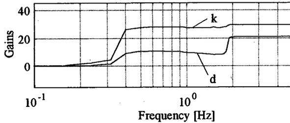
Fig. 14 Change in control gains corresponding to posture change of Fig. 10
