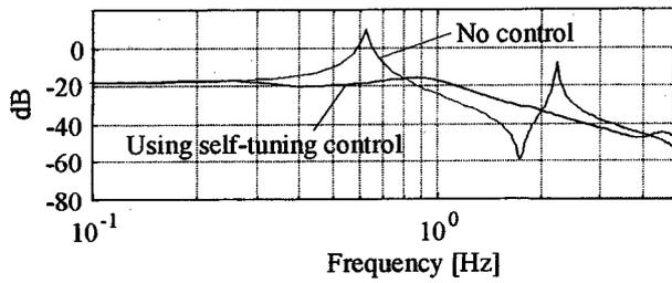
Fig. 13 Frequency response corresponding to posture change of Fig. 10
