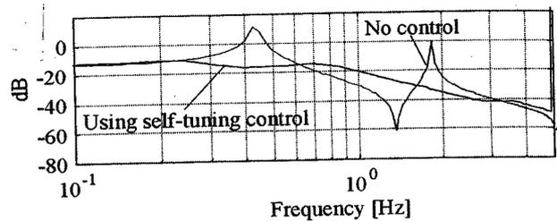
Fig. 11 Frequency response corresponding to posture change of Fig. 9
