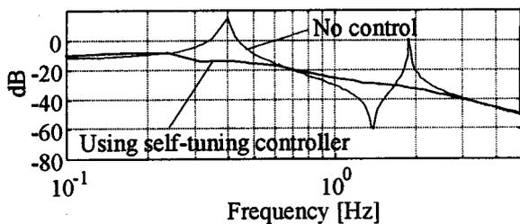
Fig. 6 Frequency response in case of self-tuning PD control
