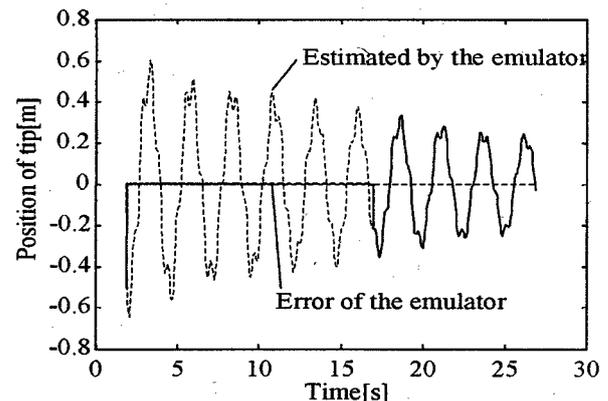
Fig. 4 Accuracy of an emulator estimating a state of the following time 1.9s
