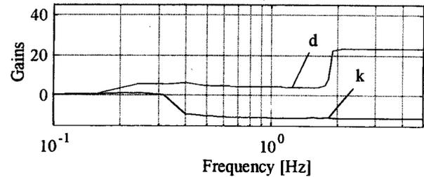
Fig. 16 Change in control gains when mass at the tip is increased
