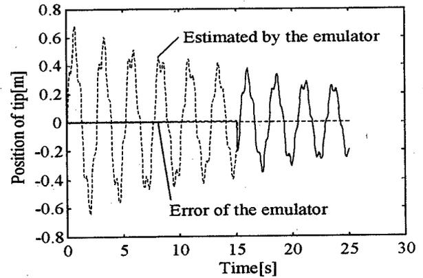
Fig. 3 Accuracy of an emulator estimating a state of the following time 0.05s
