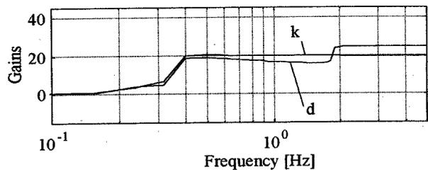
Fig. 12 Change in control gains corresponding to posture change of Fig. 9
