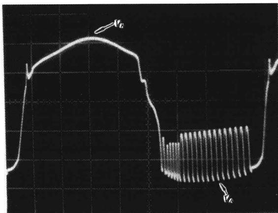
Fig. 9 Cathode Fall Waveform and Anode Fall Waveform
