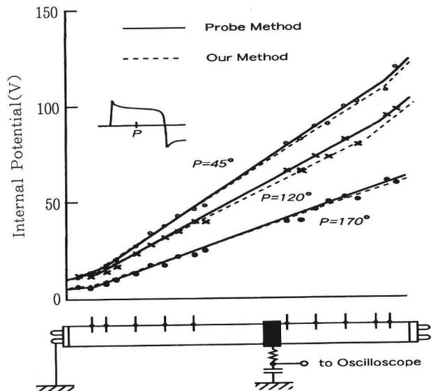
Fig. 7 Comparison of Our Method with That Using a Special Fluorescent Lamp with Internal Probes
