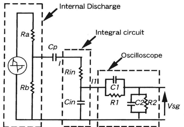
Fig. 5 Equivalent Circuit
