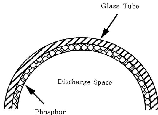
Fig. 1 Structure of Fluorescent Lamp
