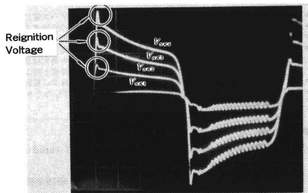
Fig. 8 Internal Axial Potential Waveform at Some Point of a Conventional Fluorescent Lamp
