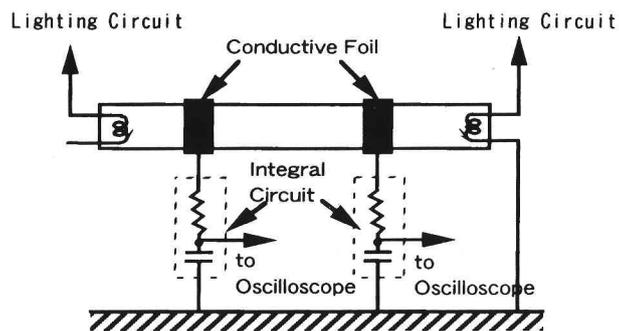
Fig. 11 Measurement Circuit for Potential Difference between Any Two Points
