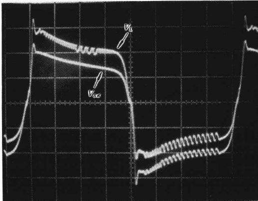
Fig. 3 Lamp Voltage Waveform and Internal Discharge Waveform
