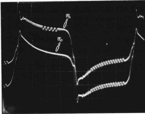
Fig. 2 Lamp Voltage Waveform and Output Signal of the Foil
