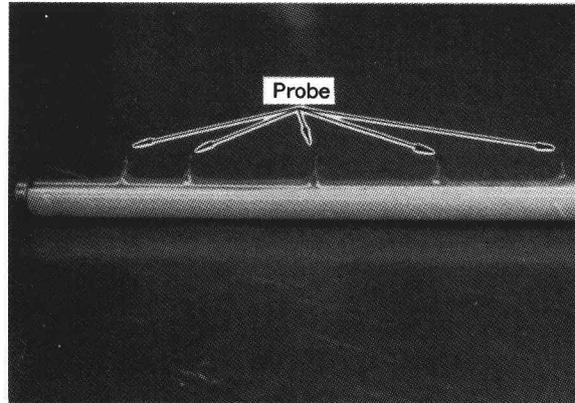
Fig. 6 Special Fluorescent Lamp with Ten Internal Probes
