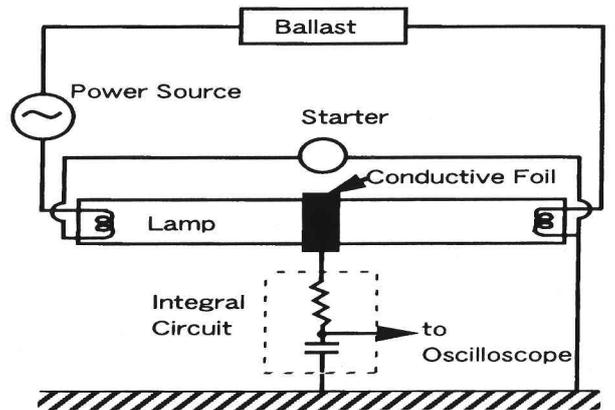
Fig. 4 Measurement Circuit
