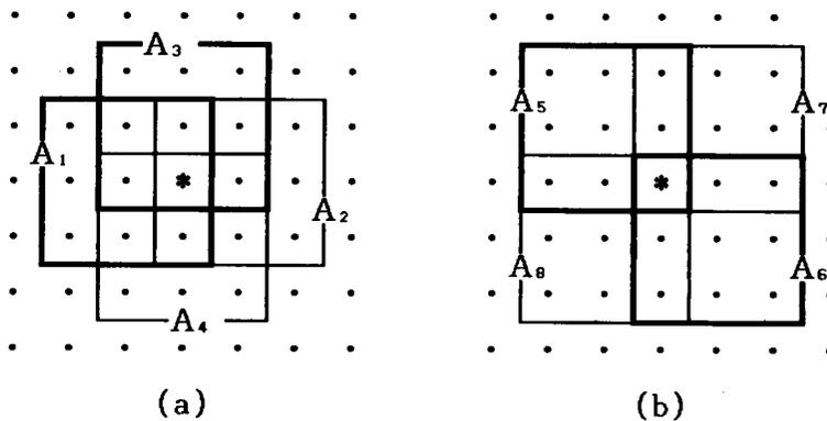
Fig. 3 The way of constructing the  $n \times n$  windows  $A_1 \sim A_8$  (for  $n=3$ ).
