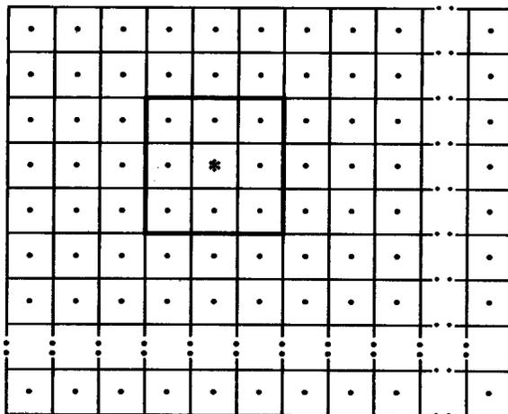
Fig. 1 Two dimensional image data and a  $n \times n$  window (for  $n=3$ ).
