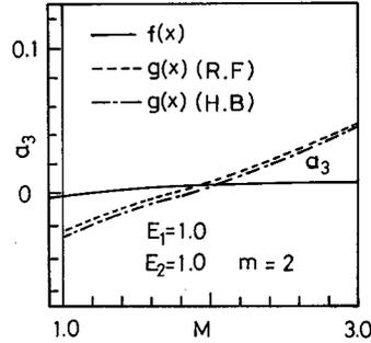
Fig. 10 Initial value responses of Fourier component  $a_3$  of harmonic solutions in case  $m = 2$
