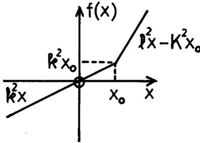
Fig. 1 Piecewise linear restoring force
