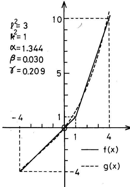
Fig. 4 Restoring force characteristics of  $f(x)$  and  $g(x)$  in case  $x_0 = 1$
