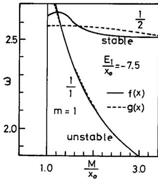
Fig. 5 Branching phenomena of solutions of order  $1/2$  from harmonic solutions in  $M-\omega$  plane in case  $E_1 = -7.5$ ,  $m = 1$ , and  $x_0 = 1$
