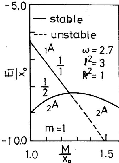
Fig. 11 Branching phenomena of subharmonic solutions of order  $1/2$  from harmonic solutions in  $M$ - $E$  plane in case the piecewise linear system
