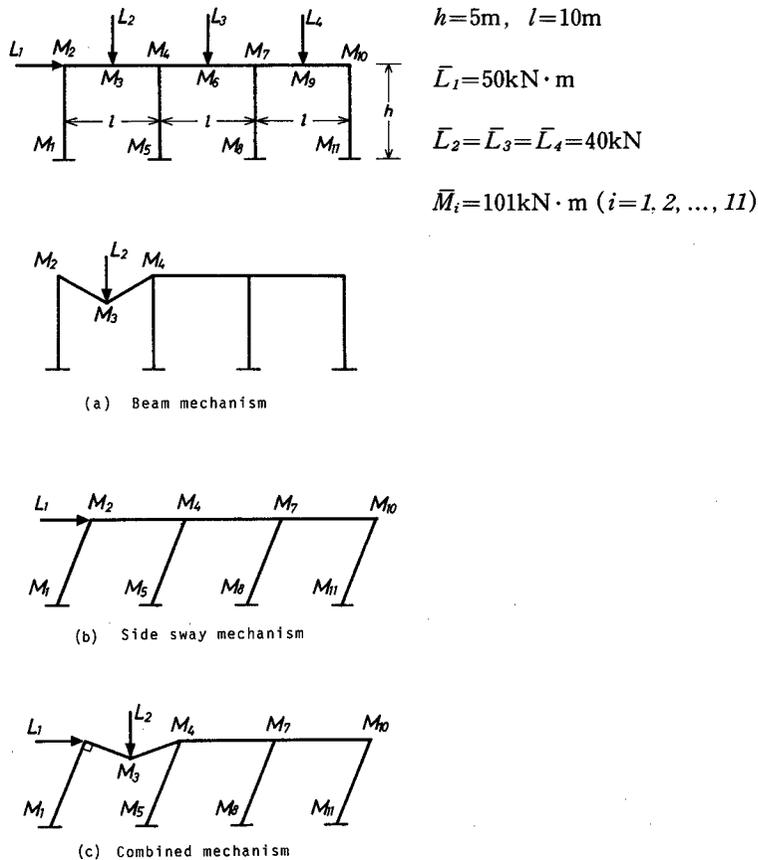
Fig. 4 Collapse modes of a three bay frame structure
