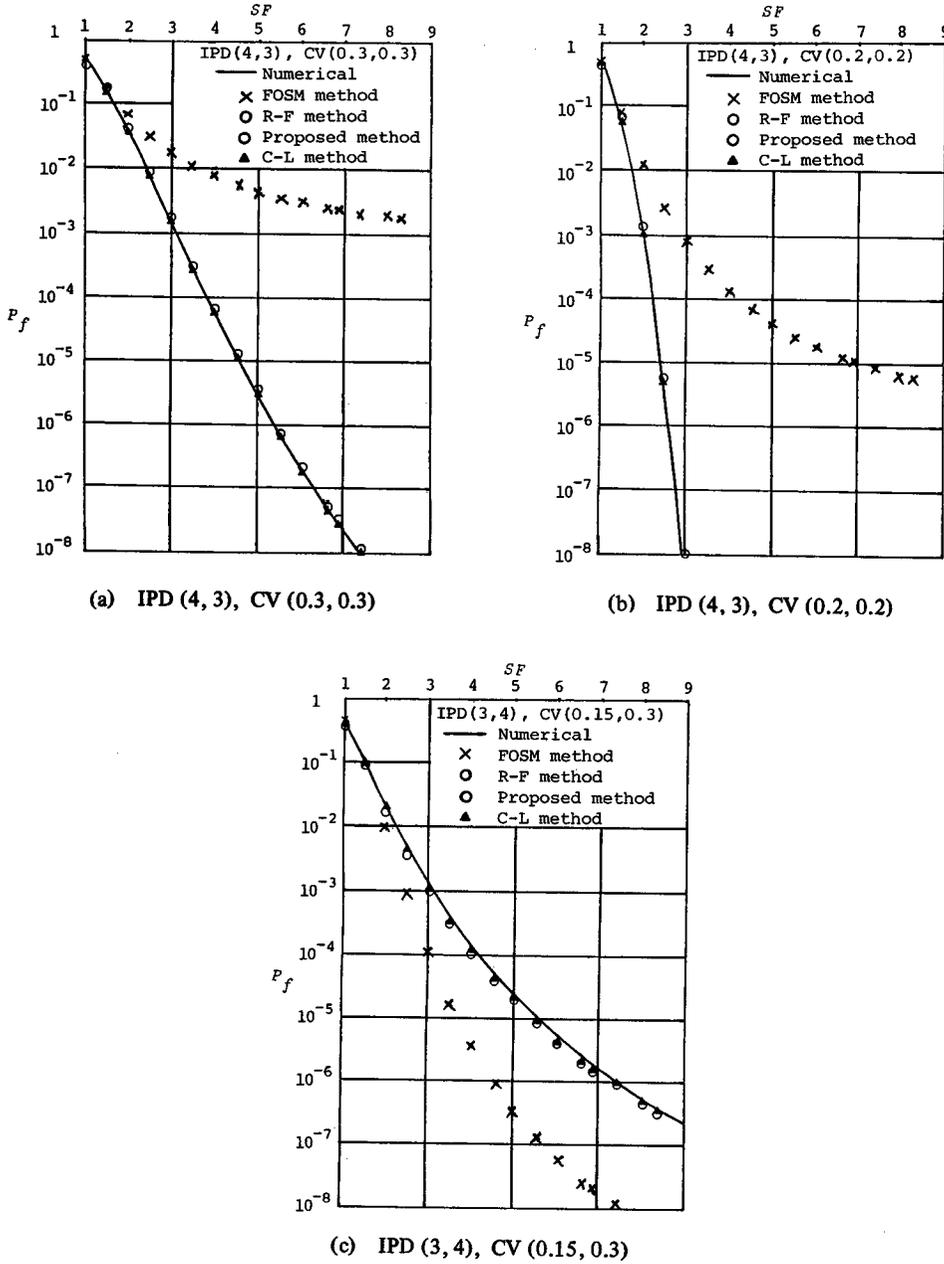
Fig. 3 Failure probability  $P_f$  versus central safety factor  $SF$  for the one-member-one-load structure
