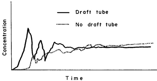
Fig. 6 Typical response curves for mixing time measurement
