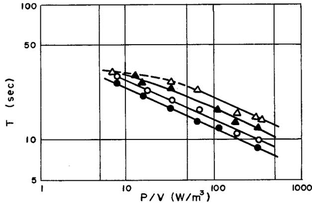
Fig. 7 Effect of  $P/V$  on mixing time  $T$ ;  $L=30$  cm,  $\Delta$ =no draft tube,  $\blacktriangle=D_d/D_t=0.10$ ,  $\circ=0.16$ ,  $\bullet=0.28$
