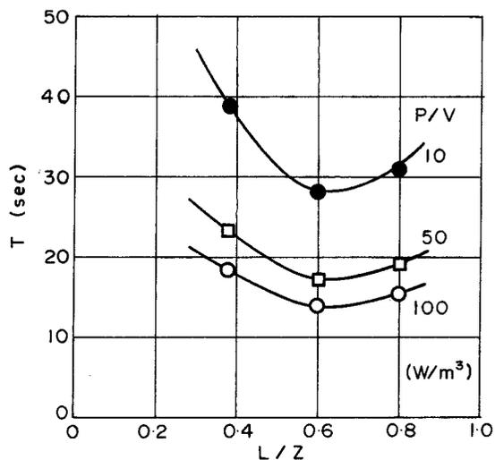
Fig. 8 Effect of draft tube length on mixing time
