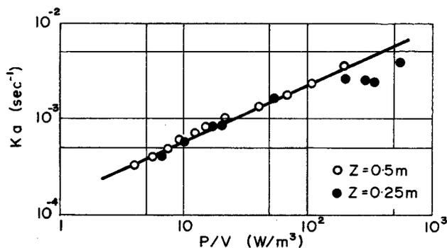
Fig. 4 Effect of power consumption per unit volume of content on the overall volumetric mass transfer coefficient;  $D_d = 8$  cm,  $H = 5$  cm,  $L = 15$  cm, — Eq. (4)
