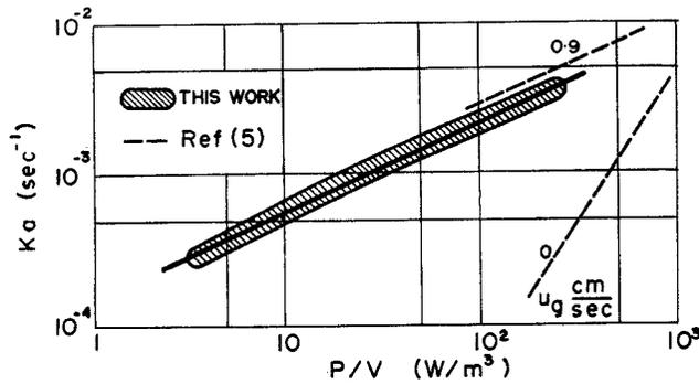
Fig. 5  $Ka$  correlation for the air-lift reactor in terms of  $P/V$ ;  $L=15-40$  cm,  $H=5-25$  cm,  $D_d=4-15$  cm,  $d_a=0.3$  cm, — Eq. (4)
