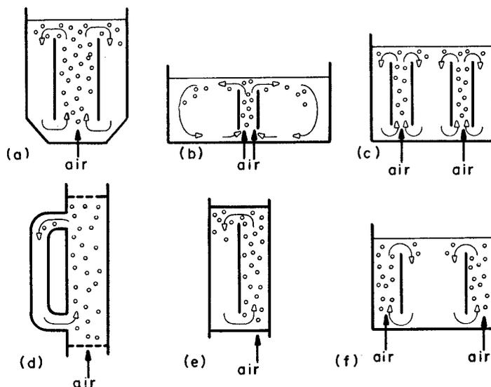
Fig. 1 Various types of air-lift equipment
