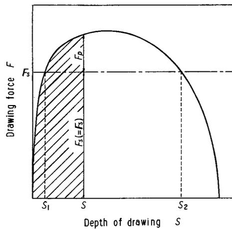
Fig. 4 Explanatory diagram for  $F$ - $S$  curve.
