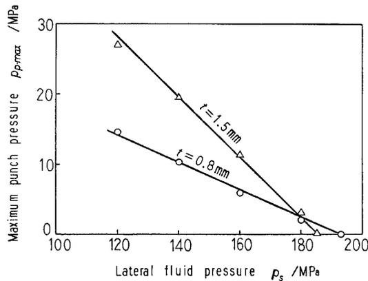
Fig. 5 Relation between lateral fluid pressure  $p_s$  and the maximum value of punch pressure  $p_{p,max}$  in  $p_p$ - $S$  curve.
