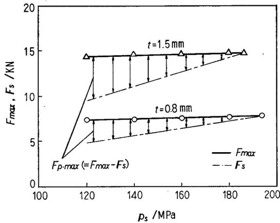
Fig. 6 Maximum drawing force  $F_{max}$  and its component  $F_s$  due to  $p_s$  ( $F_{p\cdot max}$ : component of  $F_{max}$  due to maximum punch pressure  $p_{p\cdot max}$ ).
