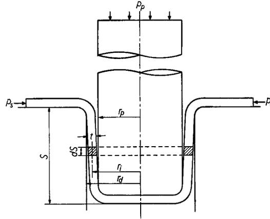
Fig. 1 Explanatory diagram for the work required to draw a blank by  $dS$  in this deep drawing process.
