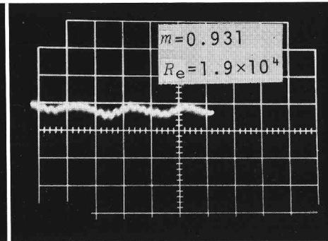
Fig. 12 Pressure signal for  $\xi=1.0$ .
