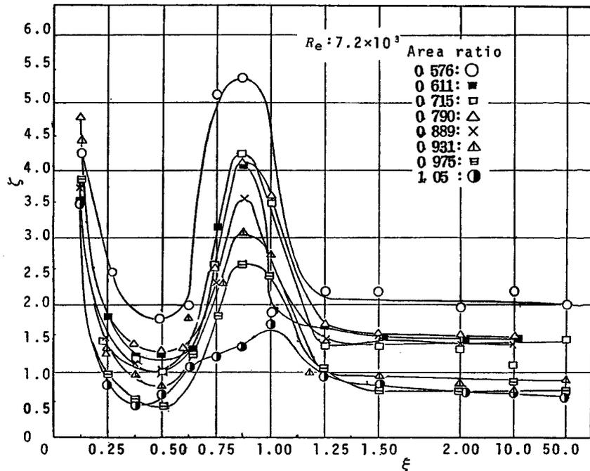
Fig. 6 Relation between loss coefficient  $\zeta$  and non-dimensional clearance length  $\xi$ .
