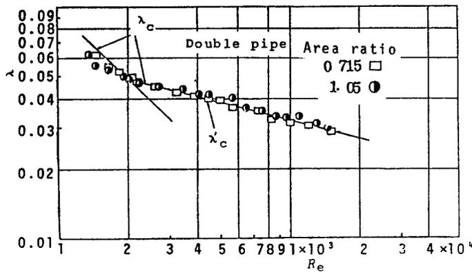
Fig. 4 Relation between friction factor  $\lambda$  and Reynolds number  $Re$ .
