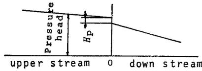
Fig. 2 Hydraulic gradient line along an inner and outer pipe.
