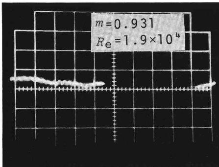
Fig. 11 Pressure signal for  $\xi=0.75$ .
