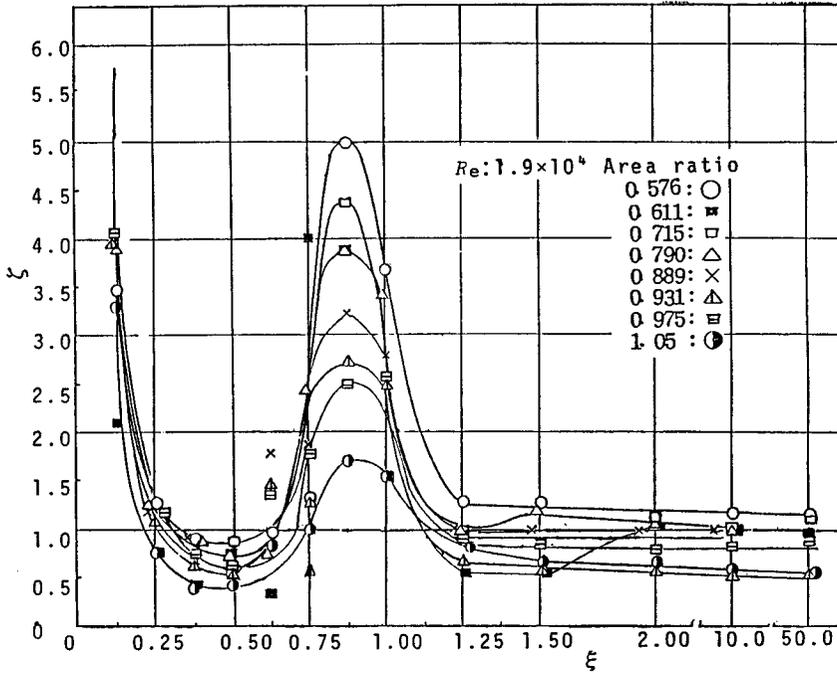
Fig. 7 Relation between loss coefficient  $\zeta$  and non-dimensional clearance length  $\xi$ .
