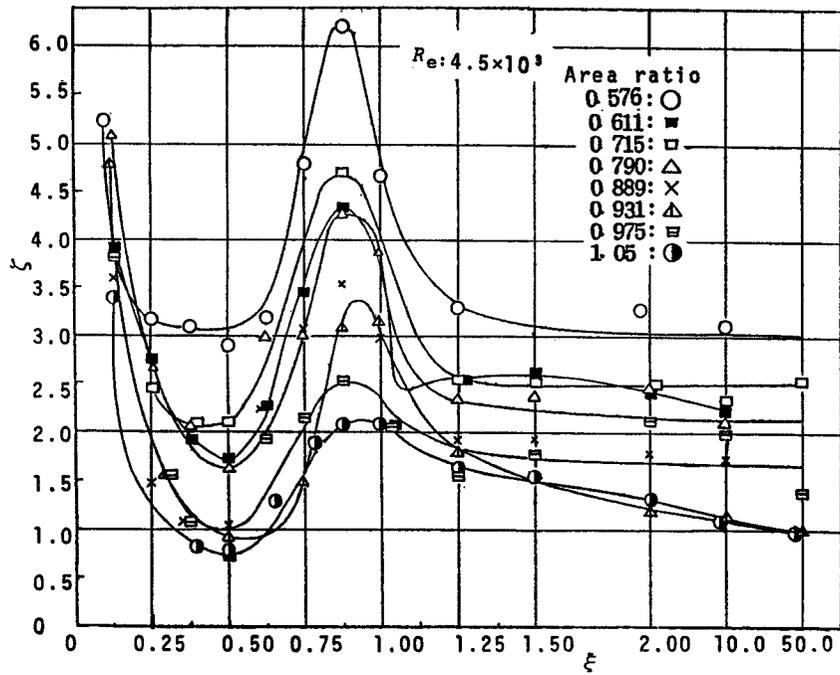
Fig. 5 Relation between loss coefficient  $\zeta$  and non-dimensional clearance length  $\xi$ .
