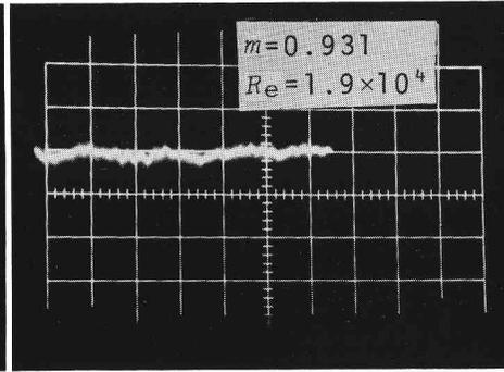
Fig. 10 Pressure signal for  $\xi=0.875$ .
