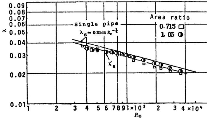
Fig. 3 Relation between friction factor  $\lambda$  and Reynolds number  $Re$ .
