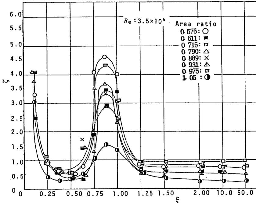
Fig. 8 Relation between loss coefficient  $\zeta$  and non-dimensional clearance length  $\xi$ .
