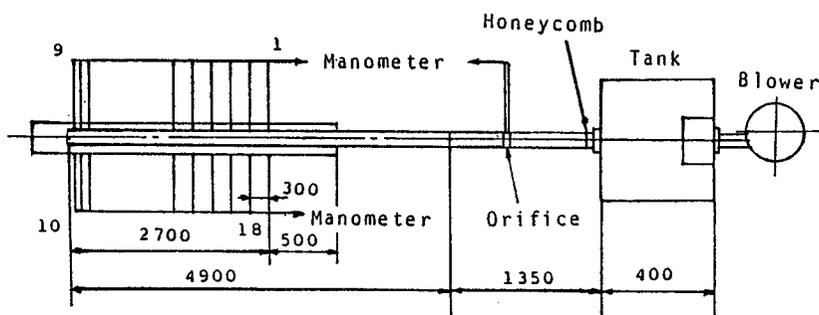
Fig. 1 Schematic diagram of complete setup of equipment.
