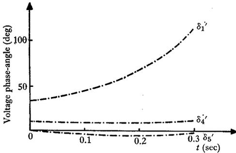
Fig. 5. Voltage phase-angles vs. time relation for the reduced system.
