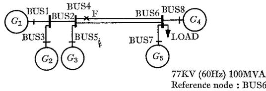
Fig. 2. 5-machine power system.
