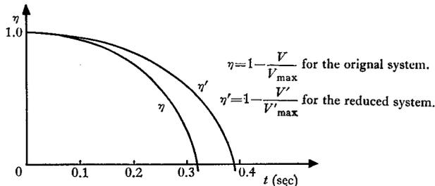
Fig. 11. Critical switching times for the original system and the reduced system.
