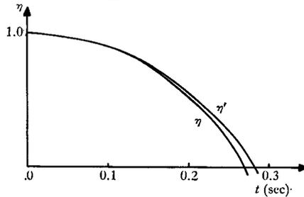
Fig. 6. Critical switching times for the original system and the reduced system.
