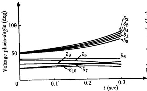
Fig. 9. Voltage phase-angles vs. time relation for the original system.
