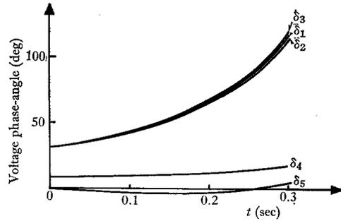
Fig. 4. Voltage phase-angles vs. time relation for the original system.
