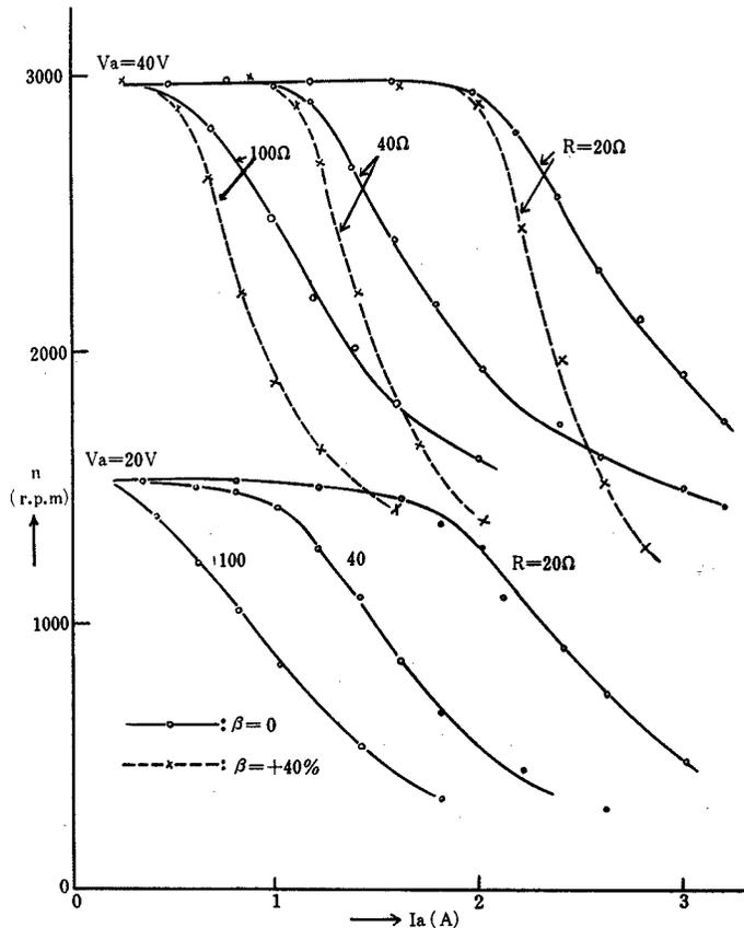
Fig. 3. Characteristics of the d-c motor operating with circuit shown in Fig. 1
