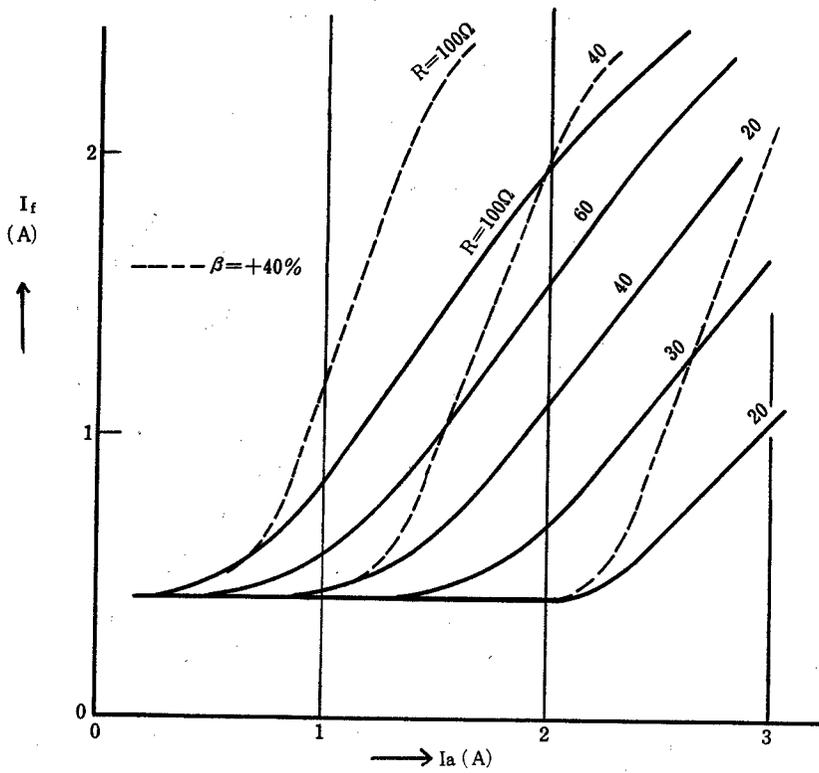
Fig. 5. Control Characteristics of m.a
