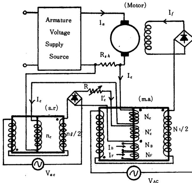
Fig. 1. Circuit construction for d-c motor having a magnetic amplifier
