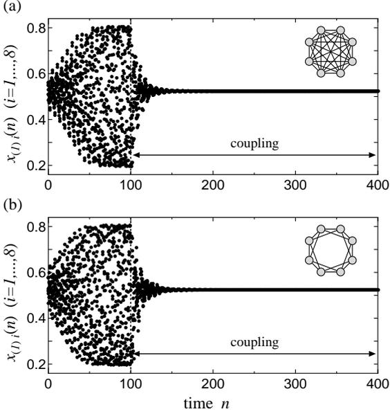
Figure 4: Time-series data of the first variables in system states  $x_i := [x_{(1)i} \ x_{(2)i}]^T$  ( $i = 1, \dots, 8$ ) with the designed parameters ( $k = 0.3$ ,  $\tau = 1$ ,  $\mathbf{b} = [1 \ 0]^T$ ,  $\mathbf{c} = [1 \ 0]$ ) for delayed logistic map (24) networks: (a) all-to-all network and (b) ring network with two nearest neighbors
