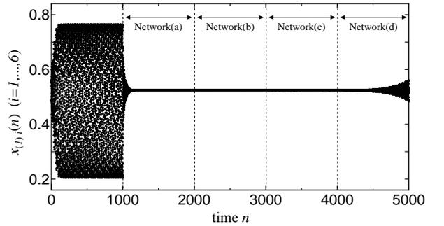
Figure 7: Time-series data of the first variables in system states  $x_i := [x_{(1)i} \ x_{(2)i}]^T$  ( $i = 1, \dots, 6$ ) with the designed parameters ( $k = 0.4$ ,  $\tau = 2$ ,  $\mathbf{b} = [0 \ 1 \ 0]^T$ , and  $\mathbf{c} = [1 \ 0 \ 0]$ ) for the four types of Henon map (25) network consisting of six maps ( $N = 6$ ) shown in Fig. 6
