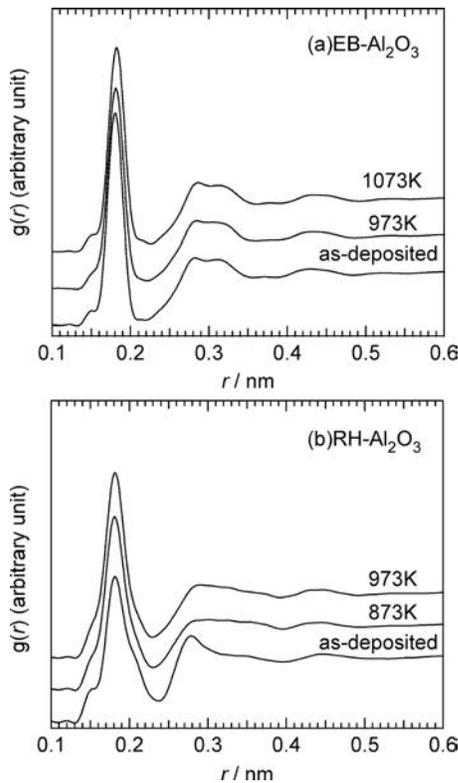
FIG. 3. PDFs of amorphous (a) EB- $\text{Al}_2\text{O}_3$  (as-deposited, 973 K, and 1073 K) and (b) RH- $\text{Al}_2\text{O}_3$  (as-deposited, 873 K, and 973 K).
