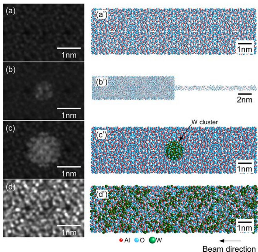
FIG. 7. (Color online) HAADF-STEM image simulations for amorphous Al<sub>2</sub>O<sub>3</sub> with a thickness of 12.3 nm. (a) Pure amorphous Al<sub>2</sub>O<sub>3</sub> with a flat surface, (b) amorphous Al<sub>2</sub>O<sub>3</sub> with a nano-pillar of 12.3 nm thick, (c) amorphous Al<sub>2</sub>O<sub>3</sub> in which W clusters with 1.5 nm are embedded, and (d) amorphous Al<sub>2</sub>O<sub>3</sub> in which W atoms are homogeneously distributed. (a')–(d') show the corresponding atomic model.
