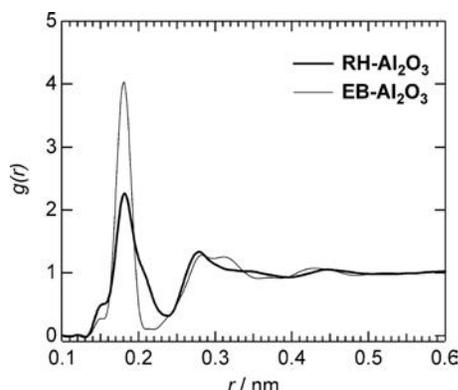
FIG. 4. Comparison of PDFs between as-deposited EB- $\text{Al}_2\text{O}_3$  and RH- $\text{Al}_2\text{O}_3$ .
