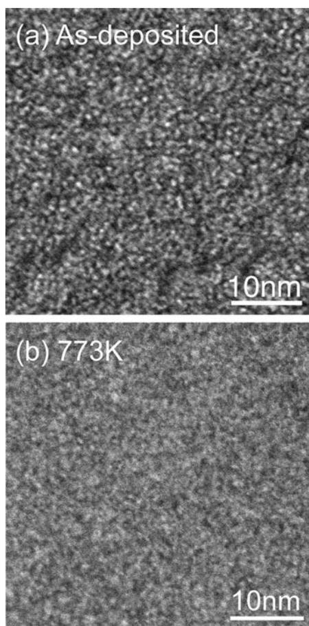
FIG. 6. HAADF-STEM images of (a) as-deposited and (b) 773 K-annealed RH-Al<sub>2</sub>O<sub>3</sub>.
