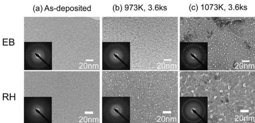
FIG. 2. BFIs and SAEDs of amorphous EB-Al<sub>2</sub>O<sub>3</sub> and RH-Al<sub>2</sub>O<sub>3</sub> before (a) and after annealing for 3.6 ks at (b) 973 K and (c) 1073 K. Reprinted with permission from R. Nakamura, T. Shudo, A. Hirata, M. Ishimaru, H. Nakajima, *Scr. Mater.*, 64/2, 198 (2011). Copyright © 2011 Elsevier.
