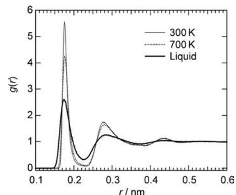
FIG. 5. MD simulations for PDFs of amorphous and liquid  $\text{Al}_2\text{O}_3$ . Solid line corresponds to amorphous  $\text{Al}_2\text{O}_3$  model at 300 K with a density of 3.34  $\text{g}/\text{cm}^3$ , dotted line to annealed amorphous  $\text{Al}_2\text{O}_3$  model at 700 K with a density of 3.29  $\text{g}/\text{cm}^3$ , and bold line to liquid  $\text{Al}_2\text{O}_3$  model at 2600 K with a density of 2.82  $\text{g}/\text{cm}^3$ .
