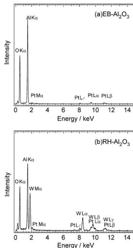
FIG. 1. EDS spectrum for as-deposited (a) EB- $\text{Al}_2\text{O}_3$  and (b) RH- $\text{Al}_2\text{O}_3$ .
