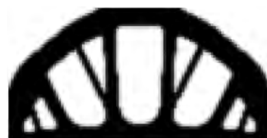
Fig. 8 Optimal configurations of the bridge example
