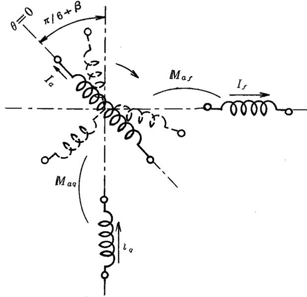
Fig. 4 Equivalent armature winding in commutation cycle.
