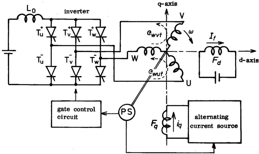
Fig. 1 Basic principle of armature-field perpendicular commutatorless motor.
