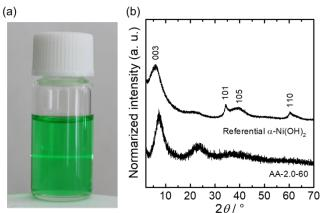
Figure 1. (a) Transparent solution of AA-2.0-60 showing Tyndall effect. (b) PXRD pattern of powder collected by drying AA-2.0-60 solution. The referential pattern was acrylate intercalated α-Ni(OH)<sub>2</sub> prepared by a standard precipitation method (see experimental section in SI).
