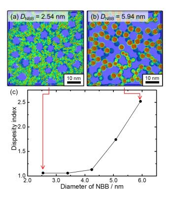
Figure 5. Typical snapshots of mesostructures formed with NBBs and F127 with  $D_{\rm NBB}=$  (a) 2.54 nm and (b) 5.94 nm. The system size of (a) is  $61.02\times61.02\times7.63~{\rm nm^3}$  and of (b) is  $68.65\times68.65\times7.63~{\rm nm^3}$ . The red spheres, green rings and blue regions are the NBB core, the interface and the F127 filled parts, respectively. (c) The change of the DI calculated from snapshots along with the
