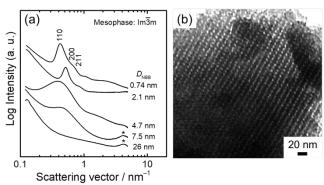
Figure 4. (a) SAXS patterns of cast-films after drying at 120 °C for 2h. The casted-films composed of  $D_{\rm NBB}=0.74$  nm, 2.1 nm, 4.7 nm, 7.5 nm, and 26 nm were prepared from F-AA-2.0-5, F-AA-2.0-60, F-AA-0.5-15, F-AA-1.0-45, and F-AA-0.1-15, respectively. \*: background peaks from  $\alpha$ -Ni(OH)<sub>2</sub> and polyimide. (b) TEM image of films prepared from AA-2.0-F-5 after heat treatment at 120 °C for 2 h and 250 °C for 2 h.
