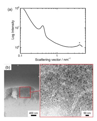
Figure 7. SAXS patterns of cast-film of Co-Cit-0.67-0.5 after drying at 120 °C for 2h. (b) Cross sectional SEM images of Co-Cit-0.67-0.5 after heat treatment at 120 °C for 2 h and 250 °C for 2 h. \*: background peaks from  $\alpha$ -Co(OH)<sub>2</sub> and/or polyimide
