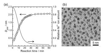
Figure 2 Time evolution of  $D_{\rm NBB}$  (open circle) and consumption of ionic Ni species (solid line) (calculated from conductivity of solution, see supporting information, SI) in the reacting solution of AA-2.0-t (t=1-60 min). (b) STEM image of AA-2.0-60 dried on a TEM copper grid.
