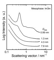
Figure 6. SAXS patterns of casted-films after drying at 120 °C for 2h. The casted-films composed of  $D_{\rm NBB}=0.99$  nm, 1.3 nm, 4.3 nm, and 7.9 nm were prepared from F-AcOH-2.0-5, F-AcOH-2.0-10, F-AcOH-2.0-30, and F-AcOH-2.0-60, respectively.  $D_{\rm NBB}$  of 4.3 nm and 7.9 nm are  $D_{\rm s}$  and their  $D_{\rm p}$  are 1.7 nm and 2.0 nm, respectively.
