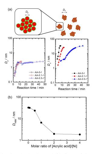
Figure 3. (a) Time-dependent growth of the diameters of primary particles,  $D_{\rm p}$  (open symbols), and secondary particles,  $D_{\rm s}$  (close symbols), prepared from AA-0-t (black), AA-0.1-t (red), and AA-0.5-t (blue) (t = 1-60). (b) Molar ratio ([AA]/[Ni]) dependence of  $D_{\rm NBB}$  ( $D_{\rm s}$  when AA/Ni  $\leq$  1.0 and  $D_{\rm p}$  when AA/Ni  $\geq$  2.0) of AA-y-30 (y = 0-4.0).
