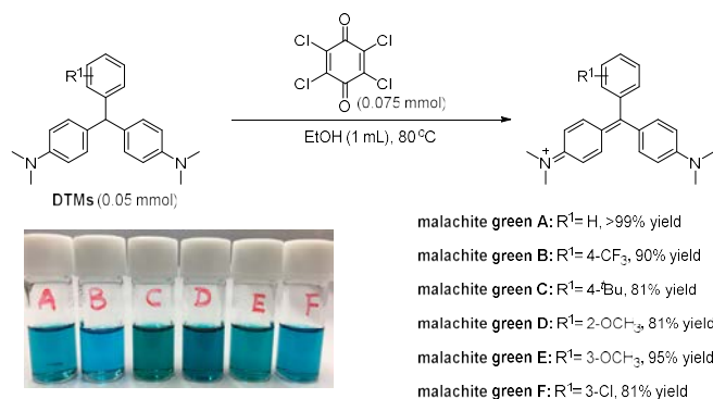
Figure 5-1. (a) Synthesis of malachite green derivatives by the oxidation of DTMs, and subsequent dissolution in CHCl 3 (50 µg/mL). Yields were determined by 1 H NMR spectroscopy using 1,3,5-trioxane as the internal standard.
