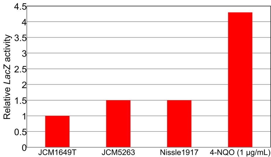
**Fig. 5** Induction of SOS response (*umuC* gene) by *E. coli* extracts in *umu* test. Relative *LacZ* activity to the *clb*<sup>-</sup> strain JCM1649T. Mean values of duplicated determinations are shown. 4-NQO as a positive control of DNA damaging agent (incubated for 3 h at 37 °C)
