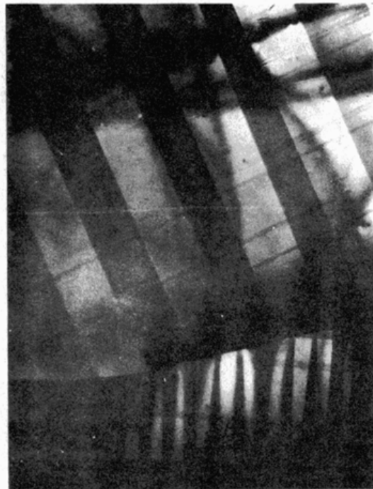
Figure 16.5. Domains in cobalt revealed by displacing the aperture and cutting out one of the components of the direct beam (From Jakubovics, unpublished work)
