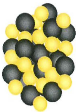
(i) Conventional composite: LiCoO 2 with no SE coating and 30 wt% SE mixing
