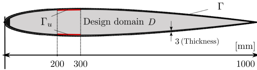
Fig. B.1: Design domain and boundary conditions for airfoils subjected to aerodynamic forces.
