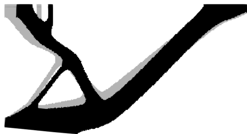
Fig. 2.10: The deformed shape of the obtained optimal solution of the compliant mechanism: The deformation is magnified by a factor of 5.
