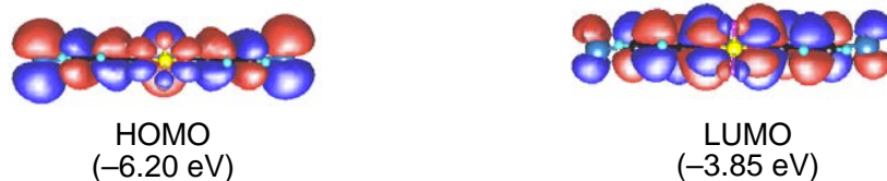
Figure 4-A7. Representation of the HOMO and LUMO of single molecule of 1hBF 2 with geometry in crystals ( M_0 ) simulated by single-point calculations using B97D method with DGDZVP and 6-311G** basis sets for iodine and for other atoms, respectively. The geometry was optimized at PW91/DNP based on results of X-ray crystallographic analyses of 1hBF 2 . Isovalue = 0.01.
