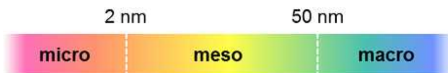
Fig. 1–1 Classification of microporous, mesoporous and macroporous materials according to porous size.
