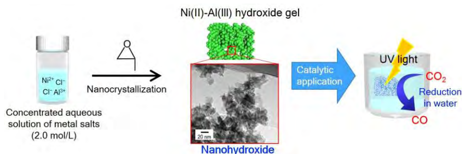
Figure 1. Schematic illustration of the synthesis and photocatalytic application of nanohydroxide. TEM image showing typical nanostructure of nano LDH prepared at Ni/Al = 2 (NLDH-2 in Table S1).
