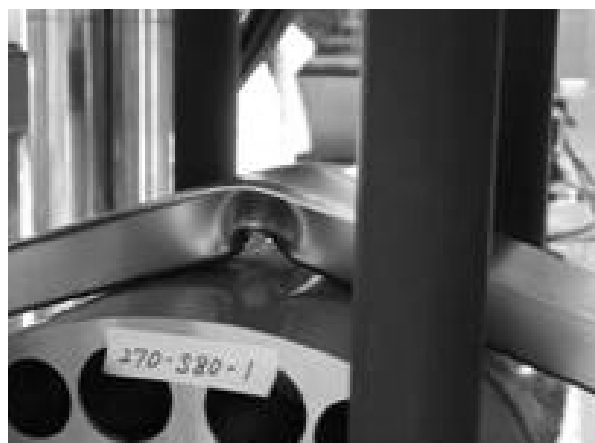
Fig.6.9 A typical deformation mode of columns just after the three-point bend test.
