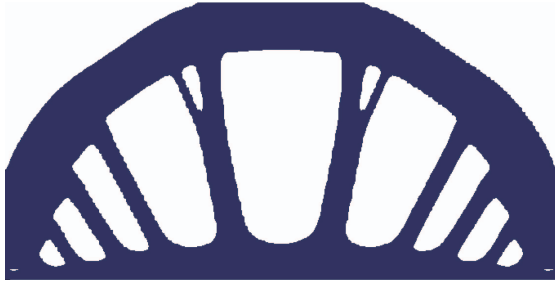
Fig. 9: Deterministic optimum configuration under uniformly distributed load condition
