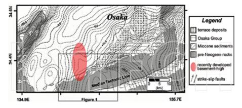
Figure 11. Regional basin morphological map of the southern Osaka Bay after Itoh et al. [20, 21]. Gravity contours are drawn at 2-mGal intervals.
