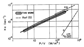
Fig. 5 Ka correlation for the air-lift reactor in terms of |P/V; L=15-40 cm, H=5-25 cm,  $D_d$ =4-15 cm,  $d_a$ =0.3 cm, — Eq. (4)
