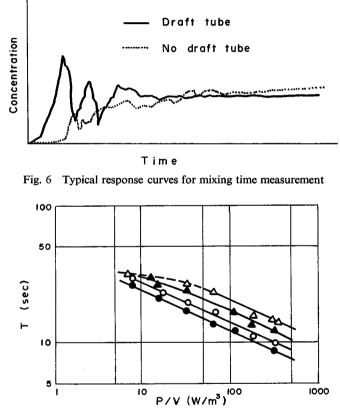
Fig. 7 Effect of P/V on mixing time T; L=30 cm,  $\Delta=\text{no}$  draft tube,  $\Delta=D_d/D_i=0.10, \bigcirc=0.16, \bigcirc=0.28$
