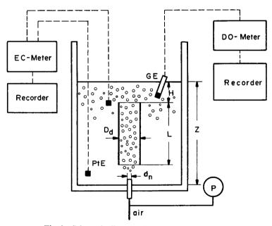
Fig. 2 Schematic diagram of experimental apparatus GE: galvanic electrode, PtE: platinum electrode, P: Bourdon-tube pressure gage
