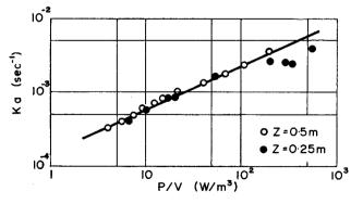
Fig. 4 Effect of power consumption per unit volume of content on the overall volumetric mass transfer coefficient;  $D_d=8$  cm, H=5 cm, L=15 cm, --- Eq. (4)
