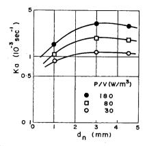
Fig. 3 Effect of nozzle diameter on the overall volumetric mass transfer coefficient
