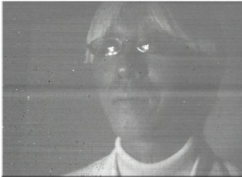
Fig. 4.15 Infrared image captured by the FPA with type-II InGaAs/GaAsSb SL absorption layer
