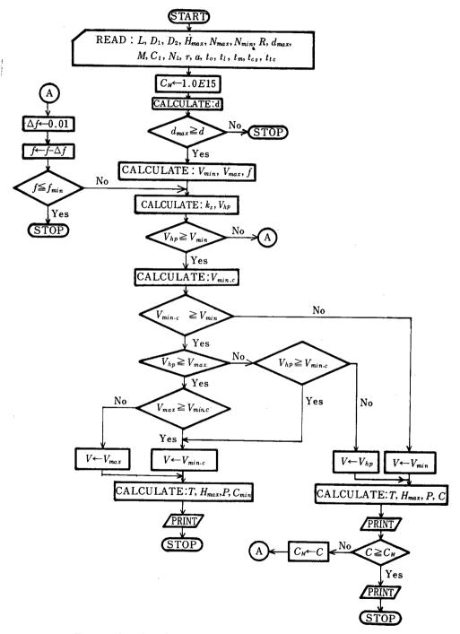
Fig. 1. Flow chart for determining the optimum machining conditions.
