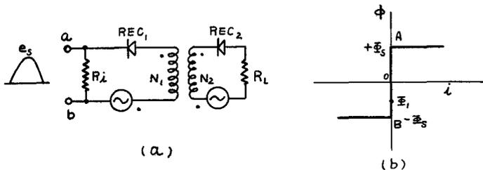
Fig. 2.1. Basic circuit of Ramey's magnetic amplifier.
