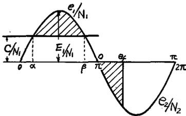
Fig. 3.1. Volt-second integral area by d-c input.
