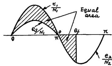
Fig. 2.2. Volt-second integral area by sinusoidal input.
