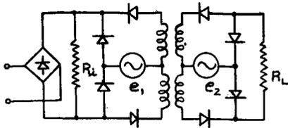
Fig. 4.1. Full wave Ramey's circuit.
