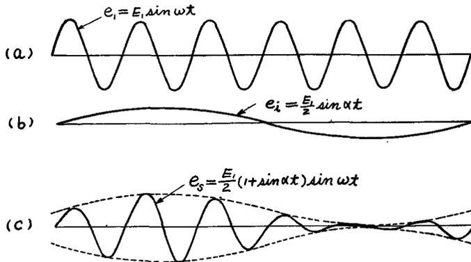
Fig. 4.2. (a) Source voltage wave form, (b) Sinusoidal signal, (c) Amplitude modulated wave.
