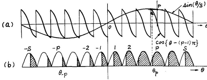
Fig. 4.3. (a) Graphical determination of firing angle.
